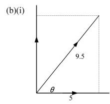
scale  $\checkmark$ 5 N and 9.5 N  $\checkmark$ correct answer  $(8.1 \text{ N} \pm 0.2 \text{ N}) \checkmark$
